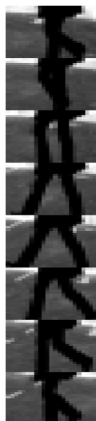
Fig. 4.13: Example of a sequence of stereo images (only the left image of each pair is shown, respectively) on which a 3D segmentation has been performed in order to determine the bounding boxes shown. The TDNN recognised the corresponding image regions as the legs of a pedestrian. Left: Example of a resulting cropped and scaled image sequence to be fed into the TDNN.
